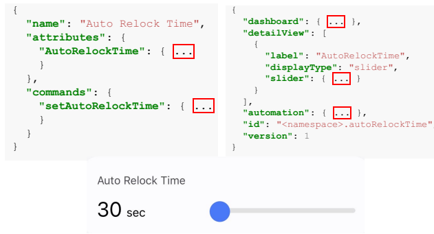
Figure 15: Example code of capability definition (upper-left) and presentation definition (upper-right). The capability view in the SmartThings app is shown at the bottom.
